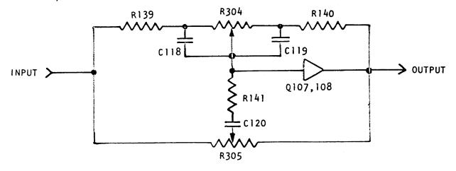
Figure 3-6A TONE CONTROL BLOCK DIAGRAM
