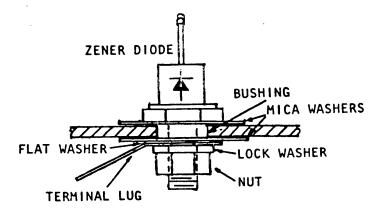
Figure 4-8 ZENER DIODE INSTALLATION
