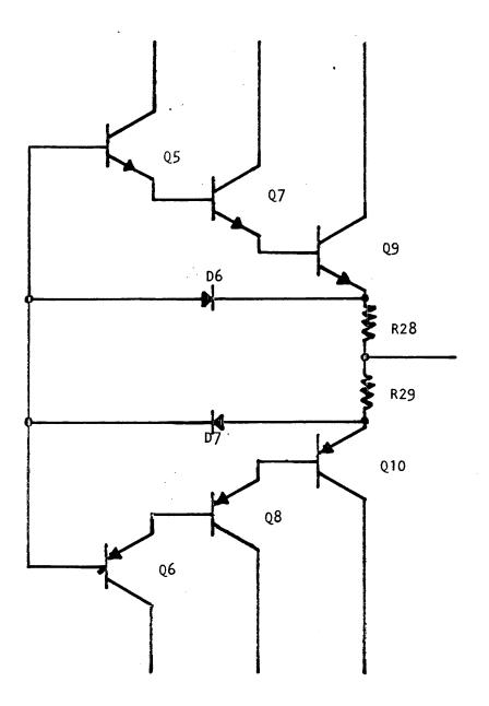
Figure 3-7 SIMPLIFIED SA660 OUTPUT AMPLIFIER
