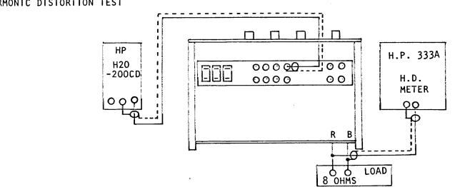
Figure 2-1 HARMONIC DISTORTION TEST CONNECTIONS
