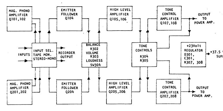
Figure 3-3 PREAMPLIFIER BLOCK DIAGRAM
