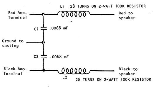
Figure 4-5 OUTPUT STAGE R. F. FILTER
