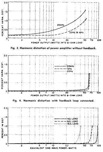
Fig. 5. Intermodulation distortion with feedback connected.
