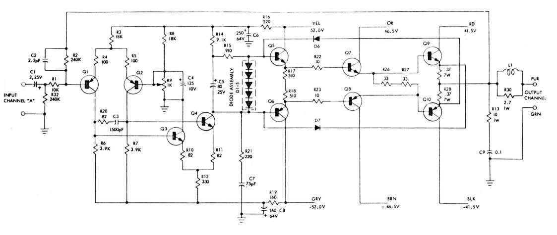
Fig. 6-25. Schematic of one channel of the J. B. Lansing SA 600 and SA 660 stereo preamp / amplifier.
